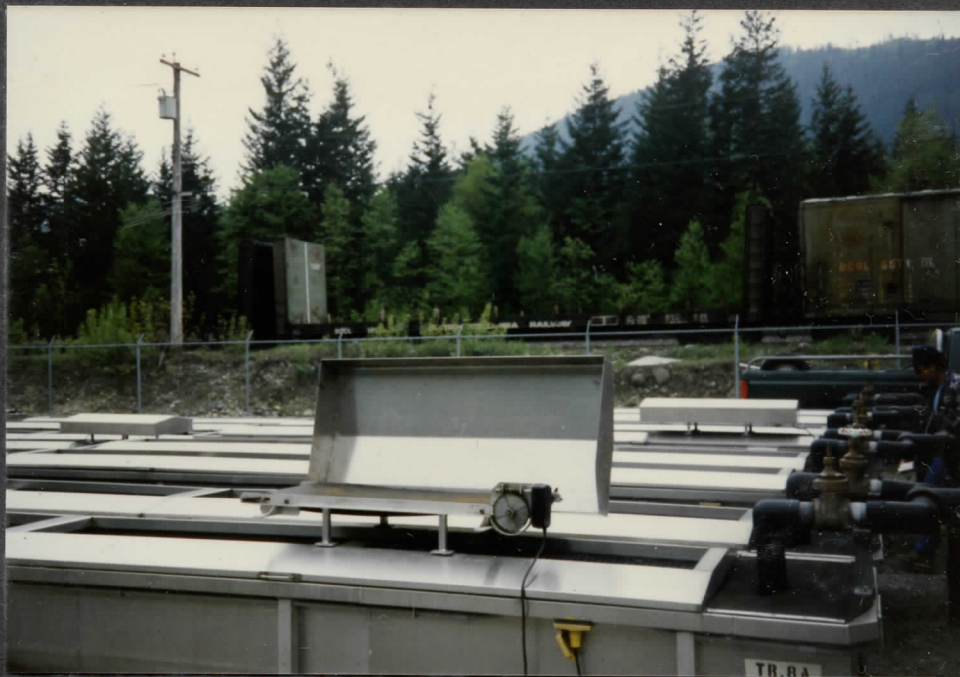
Automatic feeder used on the Cap troughs.
