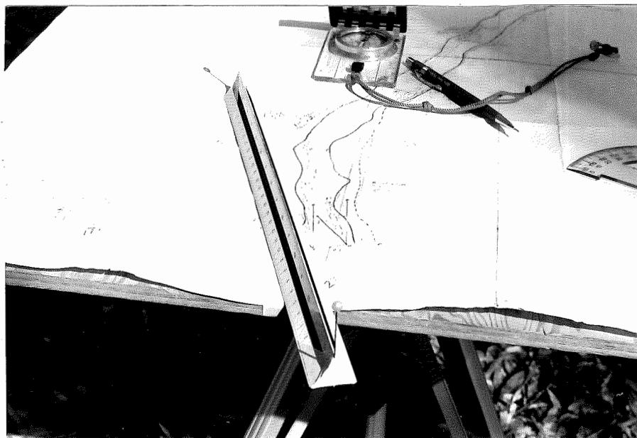
Photo 5 Ruler with pins attached, against point A and lined up with the point on shore. Note pins at each end of the baseline to help keep the ruler in place.
